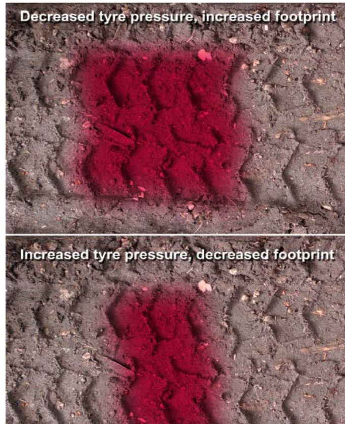
Figure 2.4 Effects of Tyre Pressure Control on road footprint. A lower air pressure can result in a contact area 60% higher than when operating under normal air pressure (Ballindalloch et al. , 2013)
