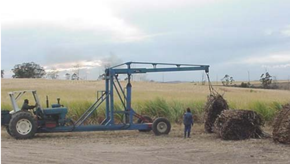
Figure 2.2 Bundled cane being loaded by a mobile derrick crane at a transloading zone (Photograph courtesy of Lyne)
