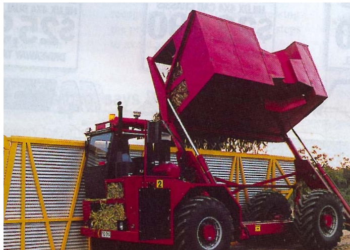
Figure 2.12 Cane being off-loaded by a hydraulic side-tipping trailer in Australia (Lyne, 2010)
