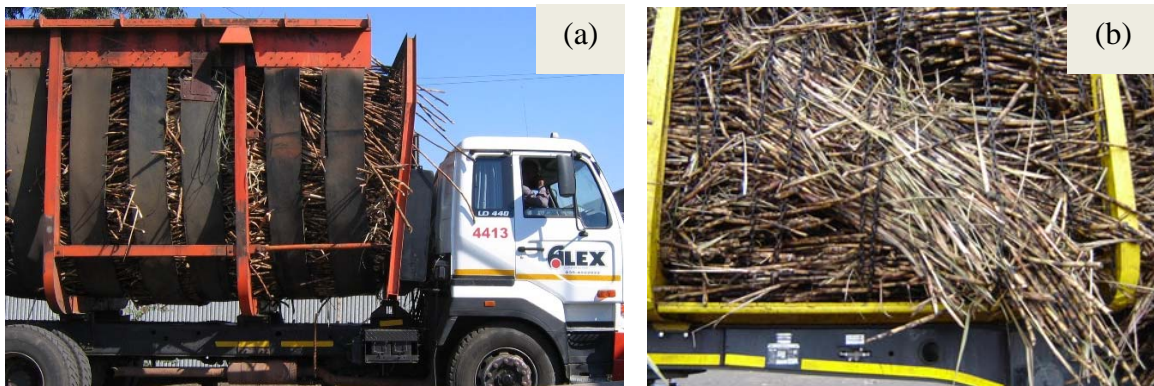
Figure 2.8 (a) Cane truck with belts in place of the chains (Lyne, 2010) (b) Overhang of cane from the side of the trailer
