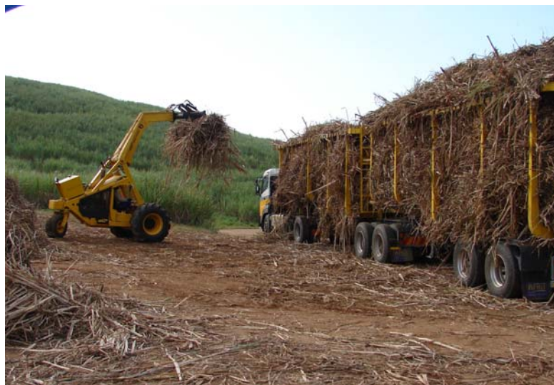
Figure 2.3 Three-wheel grab-loader loading cane at transloading zone
