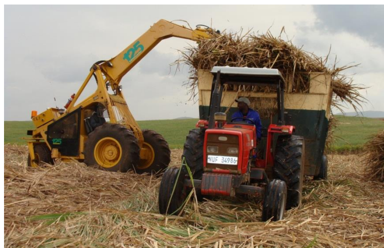
Figure 2.7 A non-slewing loader which is most commonly used in the South African sugarcane industry.
