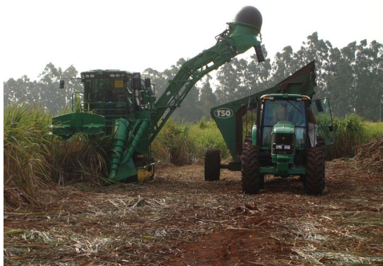
Figure 2.4 A chopper harvester and an accompanying tractor trailer to receive the cane billets.
