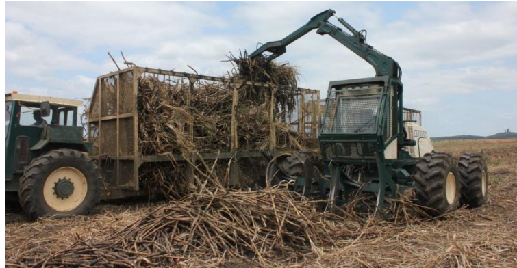
Figure 2.6 A slewing loader fitted with push-piler in the front at a wheel spacing of 3 m.
